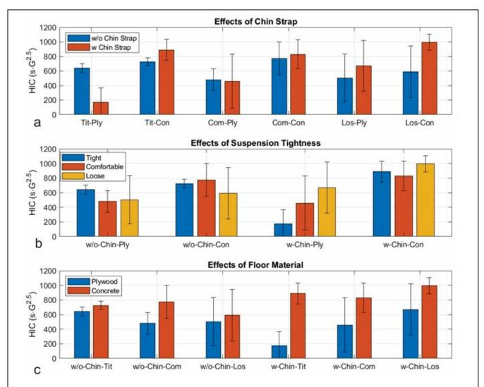
**Figure 3.** HIC<sub>15</sub> of the manikin tested in different conditions. (a) Effects of the chin strap use. (b) Effects of the suspension tightness. (c) Effects of the impact surface materials. Tit-, Com- and Los- imply the impact tests with Tight, Comfortable, and Loose suspension, respectively. W/o-Chin and w-Chin imply the impact tests without and with chin strap, respectively. Ply and Con imply the impact surface covered with plywood and concrete, respectively.
